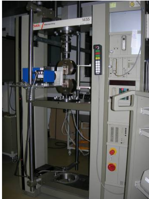
Figure 12. Machine de traction ZWICK 1455 SM
