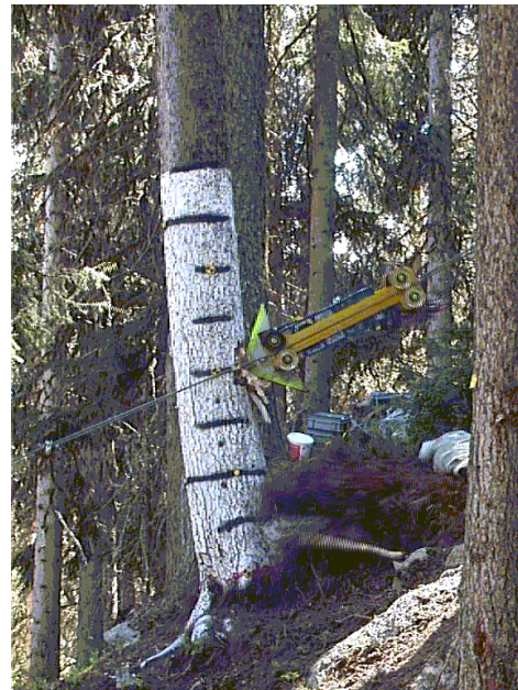
Fig. 12 Impact trolley (simulated rock, yellow) hits the tree stem. The stem base is colored white with black lines at every percent of stem height to optimize the stem tracking procedure in the image series with the Stemtrack software. Accelerometers are attached to the trolley and to the downhill side of the stem at several heights (cf. details in paper V). Animations of the reactions of the upper and lower part of the tree during the impact event can be viewed in: www.wsl.ch/forschung/forschungsprojekte/Treestability/insitu-impact_EN?redir=1 [accessed October 2008].
