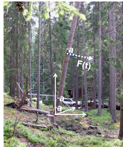
Fig. 4 The winching test involved pulling the tree sideways. The records of the pulling force F and of the stem position are made with reference to the stem base in a 3D-coordinate system and to time ( t ). Records of the stem inclination ( a ) and digital images help determine the 3D-position ( x, y, z ) of the stem while pulling, where z is the height and x is the azimuth of the pulling direction.
