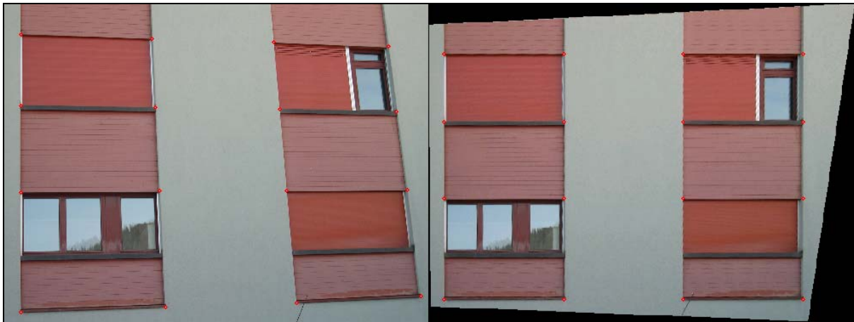
Fig. A2- 13: Spatial referencing/rectification of image: original photo (left panel); referenced images (right panel). The image, which was taken with set-up B 14 in Fig. A2- 12, includes 16 visible red markers.
