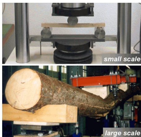
Fig. 11 Bending tests in the laboratory of small-scale samples with rectangular cross sections (top) and of entire stem sections (bottom).
