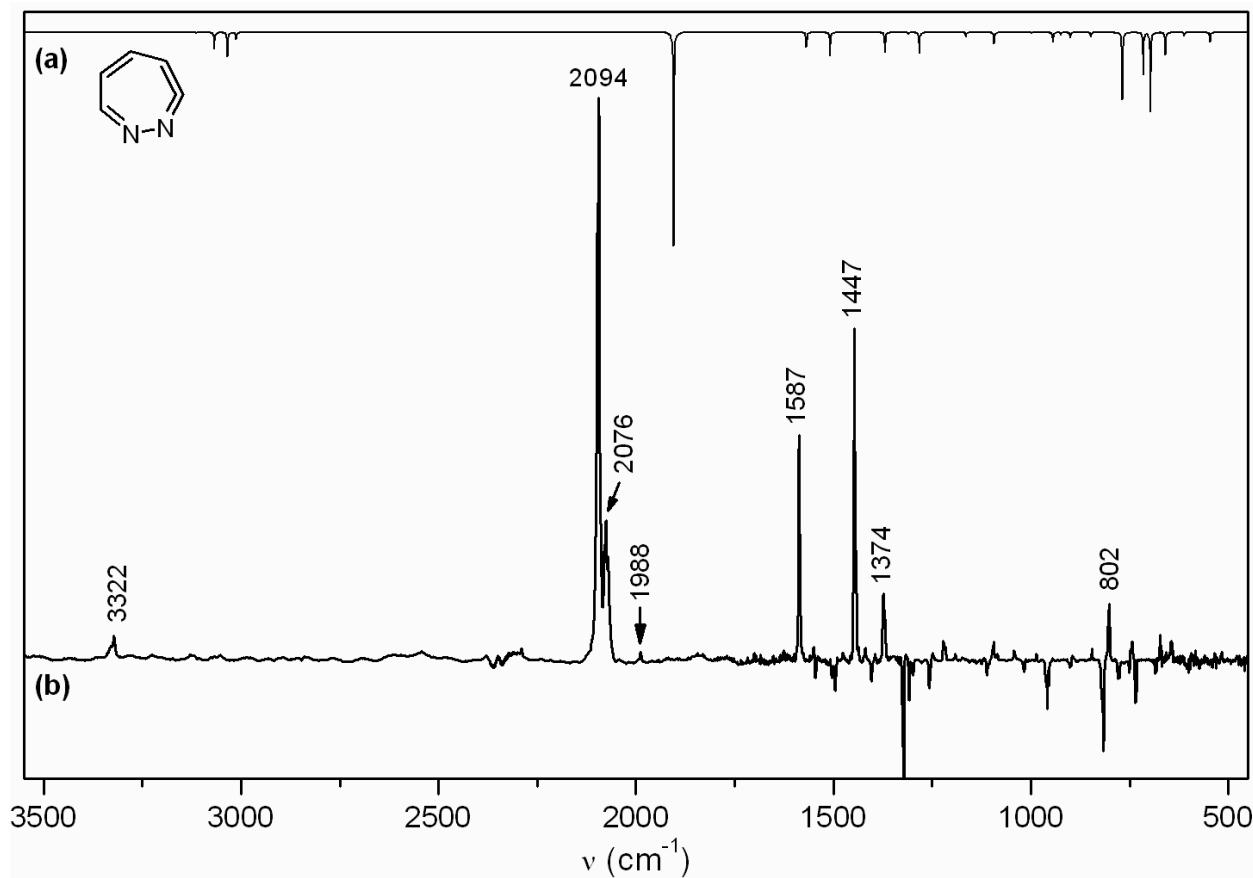
**Figure S14.** (a) Calculated spectrum of ketenimine **17** at the B3LYP/6-311G\*\* level, wavenumbers scaled by 0.967. (b) Ar matrix IR spectrum resulting from photolysis of triazolopyridazine **8** at 222 nm for 2 min, showing prominent presence of diazo compounds and absence of **17**.
