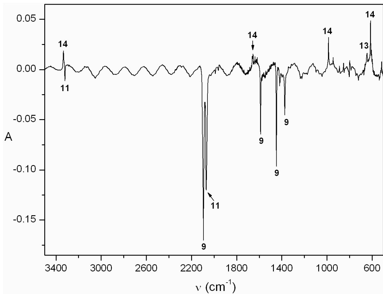
**Figure S6.** Matrix IR spectrum from photolysis of a mixture of diazo compounds **9** and **11** at 281 nm (interference filter) for 20 min (positive peaks, **14** and a trace of **13**), after initial photolysis of triazole **8** at 254 nm for 4 h (negative peaks, a mixture of **9** and **11**). The photolysis at 281 nm apparently does not touch the triazole **8** which has minimum absorption in the UV spectrum at 281 nm (Figure S1).
