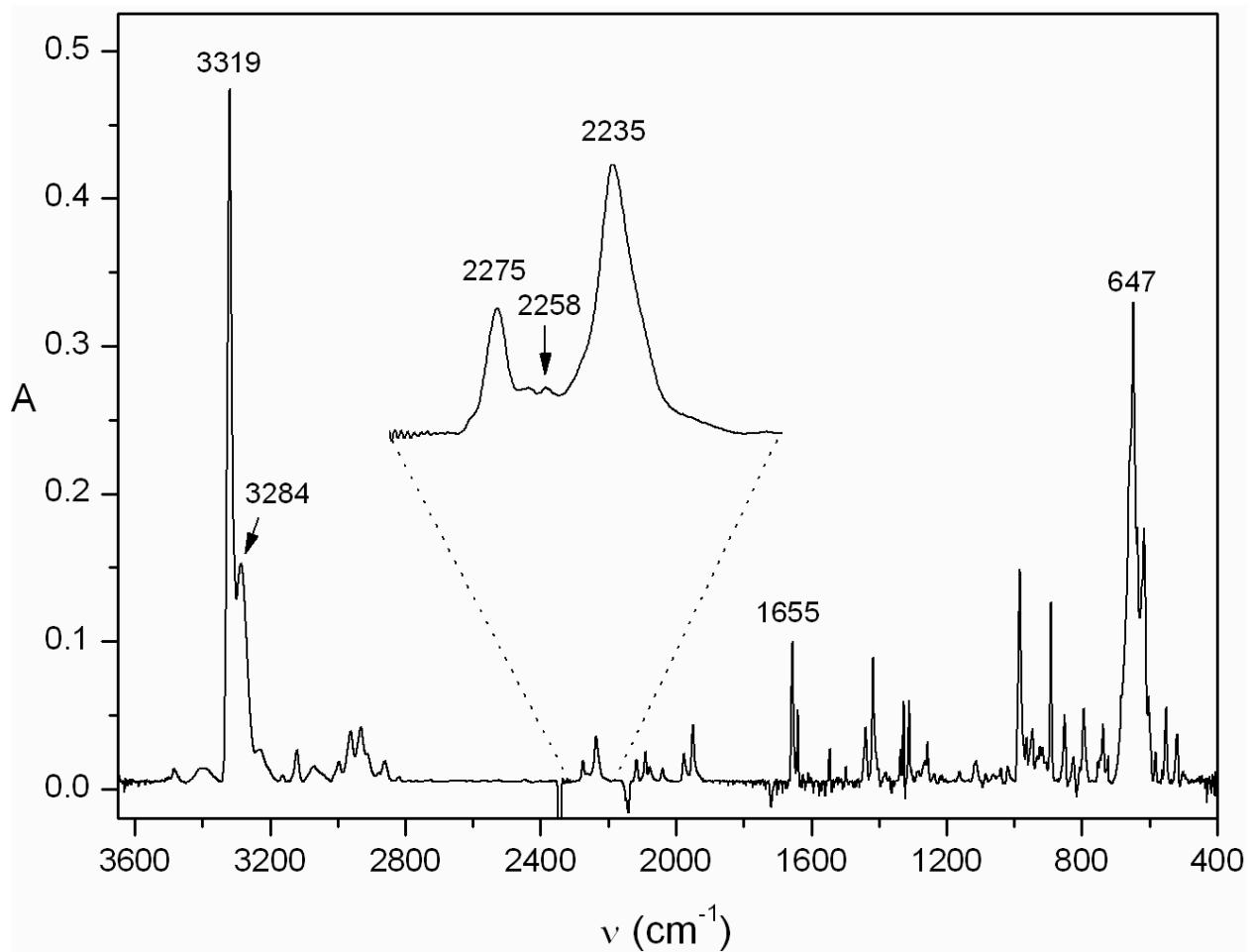
**Figure S9.** Ar matrix IR (difference) spectrum obtained from the FVT of **8** at 700 °C, showing CN peaks of glutacononitrile (2275 and 2235  $\text{cm}^{-1}$ ), 2-cyanopyrrole (2235  $\text{cm}^{-1}$ ), and 3-cyanopyrrole (2260  $\text{cm}^{-1}$ ). The absorption at 3284  $\text{cm}^{-1}$  is probably due to NH stretches in cyanopyrroles. The strong band at 3319-3333  $\text{cm}^{-1}$  is due to acetylenes **13-15**.
