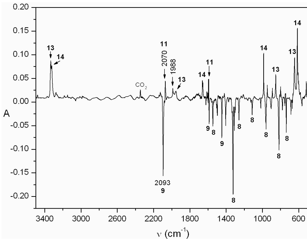
**Figure S5.** Ar matrix IR spectrum from prolonged photolysis of triazole **8** at 254 nm (low pressure Hg lamp). Positive peaks, a mixture of **11**, **13** and **14** after photolysis for 7 h. Negative peaks, a mixture of **9** and **8** after photoysis for 5 h. The positive peak at  $1988 \text{ cm}^{-1}$  is possibly due to cyclic carbodiimide **21** (see text).
