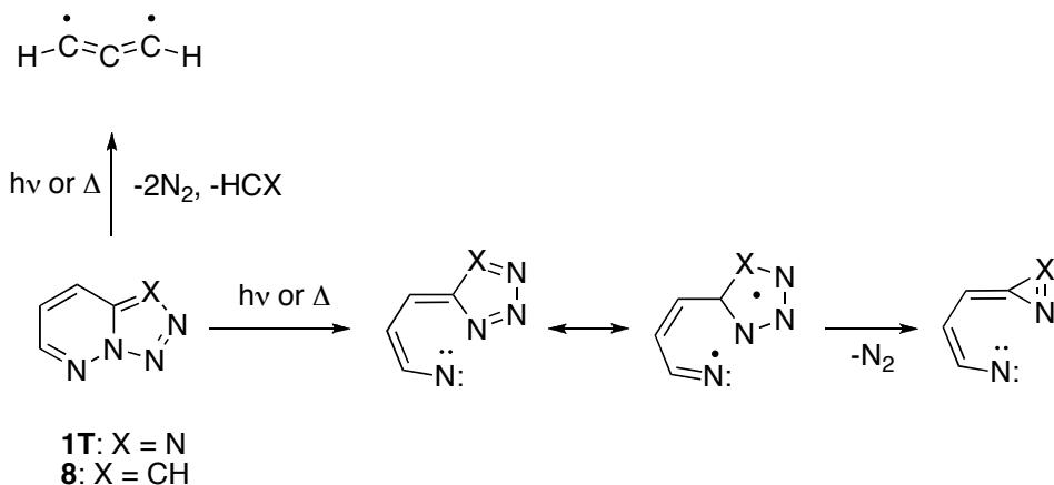
**Scheme S1.** Potential carriers of the major triplet signal B ( $X_2 = 5956$ ;  $Y_2 = 5986 \text{ G}$ ) in Figure S4, which is formed on matrix photolysis of **8** and either FVT or photolysis of **1T**.
