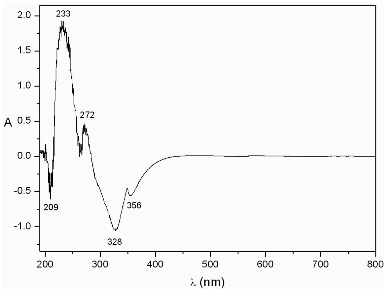
**Figure S11.** Difference UV spectrum obtained after photolysis of tetrazolopyridine **22T** in Ar matrix at 222 nm for 30 min (not shown), followed by 308 nm (30 min). Negative bands belong to diazacycloheptatetraene **21**. The product band at 233 and 272 nm are assigned to spiroazirene **25**, in relation to the corresponding matrix IR spectrum shown on Figure 7.
