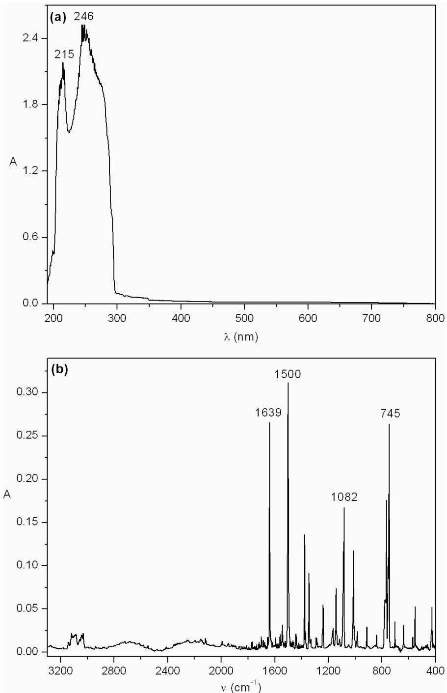
**Figure S12.** (a) Difference UV spectrum of tetrazolo[1,5-*a*]pyridine **22T** (Ar, 7K), and (b) its corresponding matrix IR spectrum, obtained from sublimation of **22T** at 80 °C ( $8 \times 10^{-6}$  mbar).
