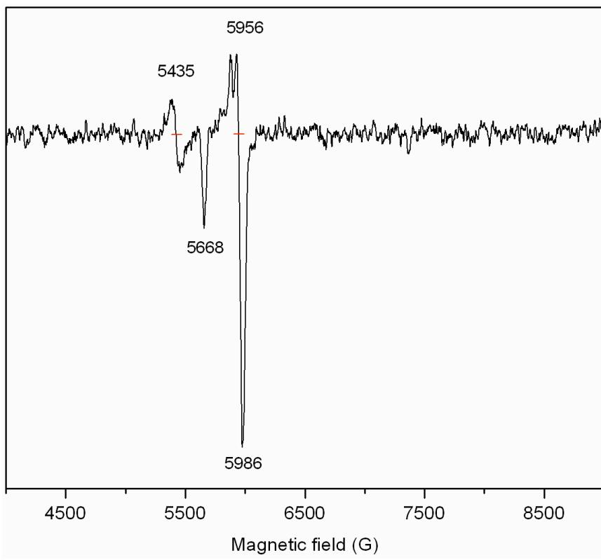
**Figure S4.** Difference ESR spectrum of unassigned triplet species after photolysis of **8** at 308 nm for 7 min (not shown) and 222 nm for 30 min. Ar matrix, 10-15 K.
