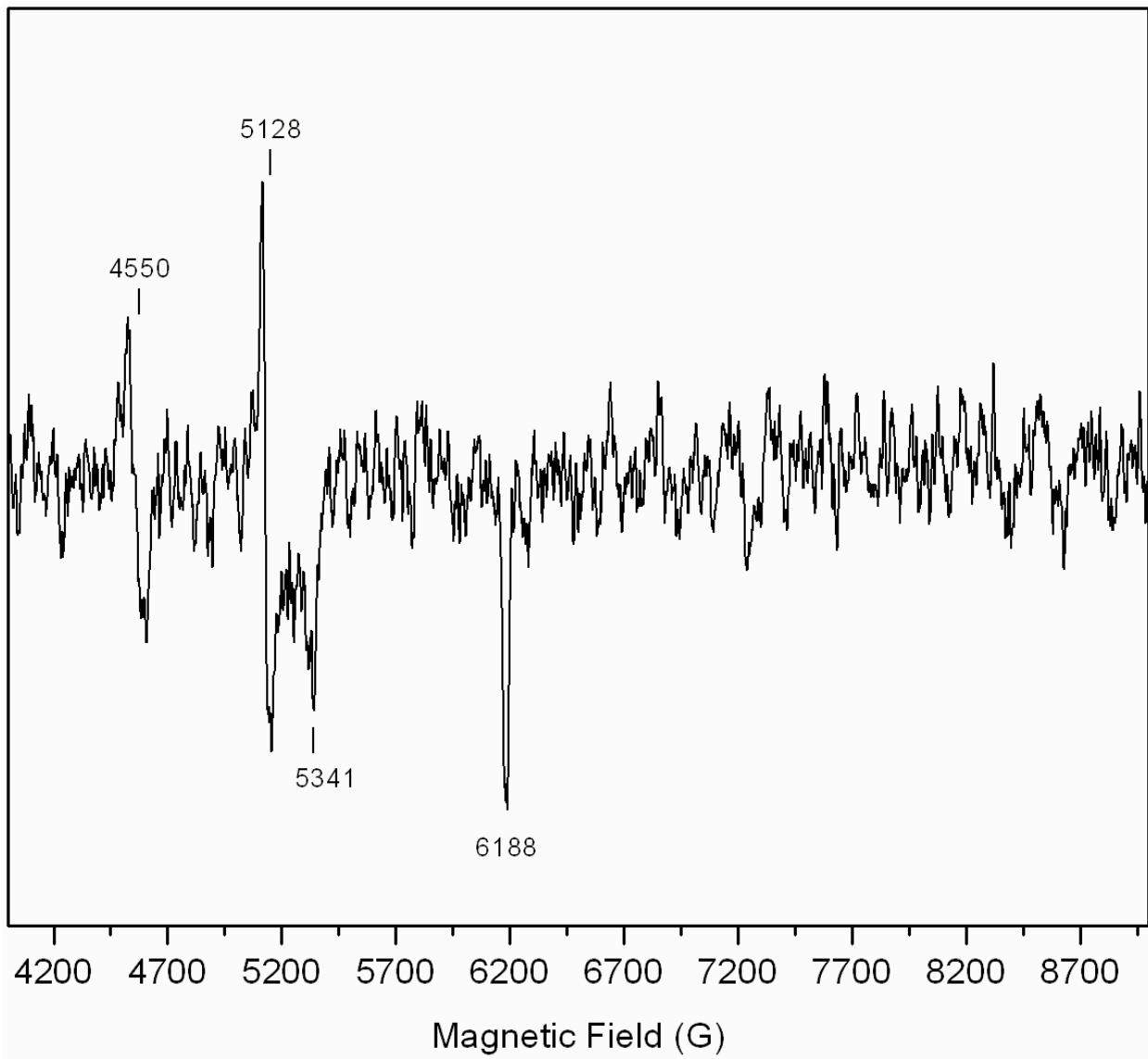
**Figure S3.** ESR spectrum obtained after 45 s of photolysis of **8** at 308 nm in Ar matrix (the spectrum is an early stage of the experiment described in Figure 3). The peaks are weak at short photolysis times, but the spectrum shows the presence of **10** (5128, 6188 G) and only one isomer of **12** (4550 ,5341 G)..
