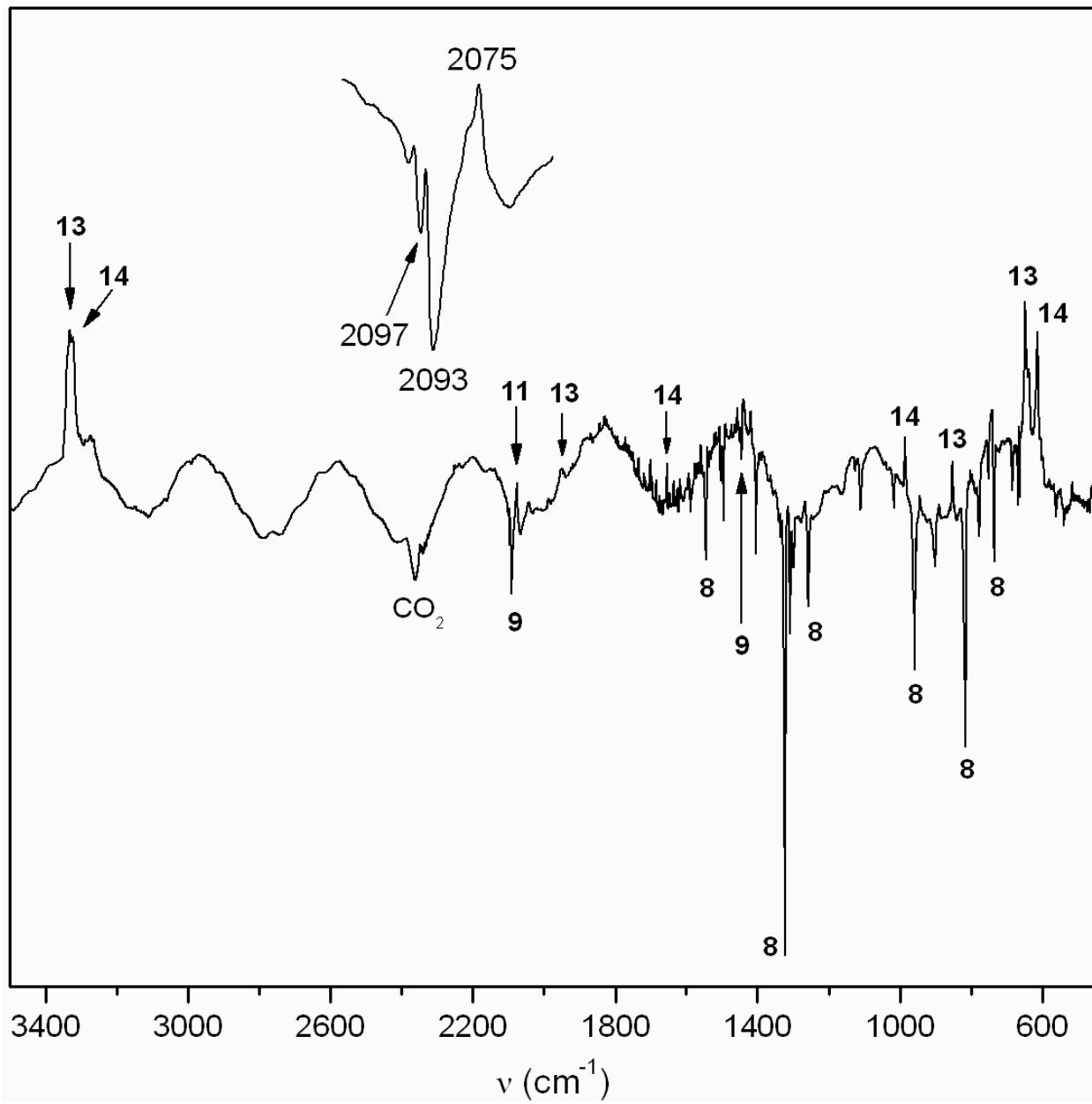
**Figure S2.** Difference IR spectrum showing a mixture of **11** as well as **13** and **14** (positive peaks), formed at the expense of triazole **8** and **9Z,E** (negative peaks), obtained by photolysis of **8** at 222 nm for 40 min. This spectrum is consistent with the order of photolysis **8** → **9** → **11** → **13/14**.
