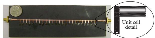
FIGURE 11: Microstrip CRLH transmission line implemented by means of shunt connected grounded stubs and interdigital capacitors. Photo courtesy by C. Caloz.
