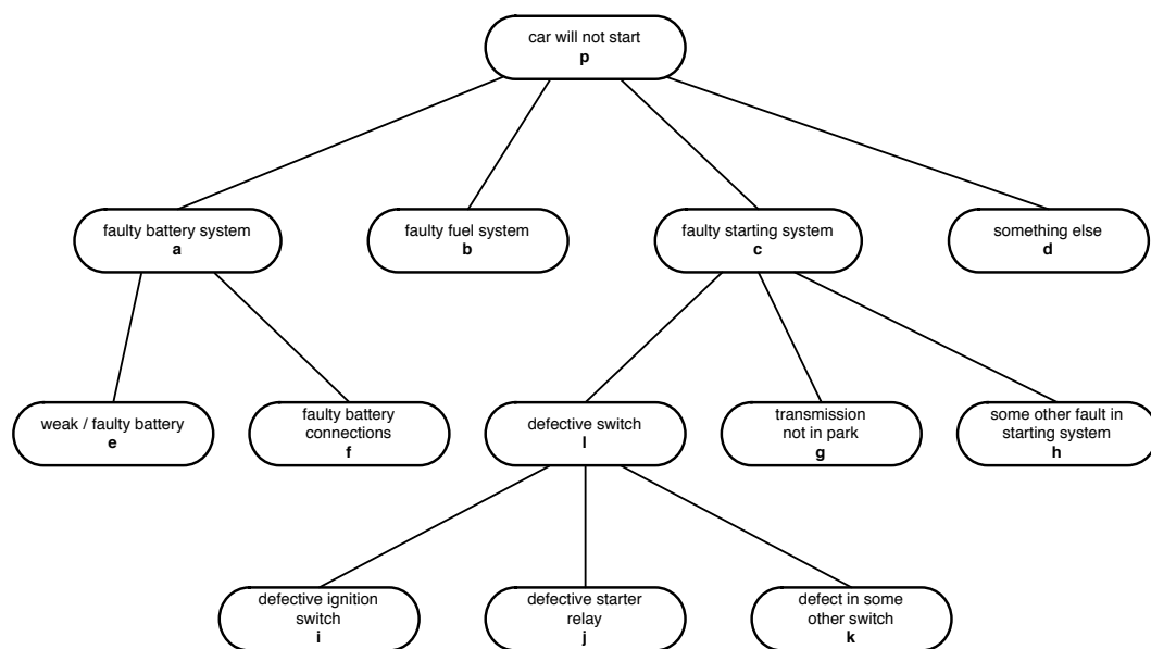
Figure 3.1: A tree of diagnoses for the “car will not start” problem
