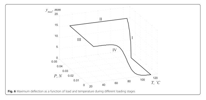
stage 1). The increase in load leads to buckling and a further nonlinear increase in deflection.
