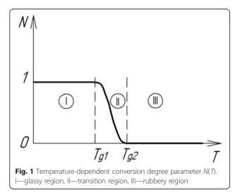
at a decreasing temperature is specified by the growth of the mechanical rigidity due to a gradual decrease in the segmental mobility and an increase in the energy of the intermolecular interactions.
