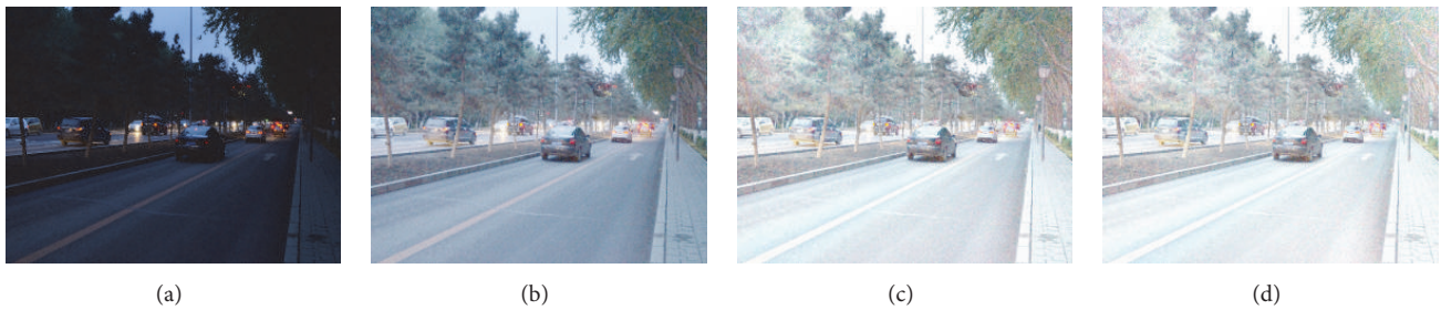
FIGURE 19: The comparative results of nighttime images with different algorithms. From left to right, respectively, the following are represented: original image, result image of the SSR, result image of Frankle-McCann, and result image of McCann99.
