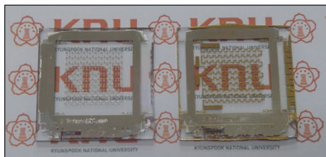
FIGURE 4: Photograph of a compact a-Si solar module for high-voltage power supply applications. It indicates the semitransparent characteristics of the individually micropatterned a-Si solar cells (left) and those serially interconnected with gold electrodes (right).
