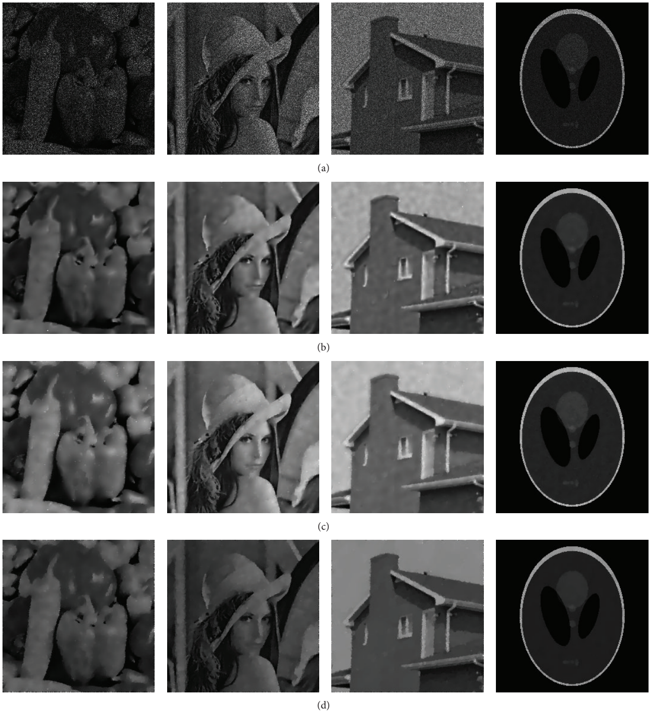
FIGURE 3: Denoising results of different methods. (a) shows the noisy images. From left to right, the noise is indicated by L = 3, 9, 15, 21 , respectively; from (b) to (d), the results are obtained by the proposed method, the TGVSNR method, and the NRSNR method, respectively. Note that all of the denoising results are generated when they reach the highest SNR of their corresponding denoising methods.
