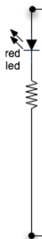
Figure 5.7: Circuit for the red led which indicate that the system is powered on
