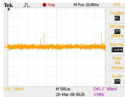
Figure 46 Stability of the regulated 12V voltage
