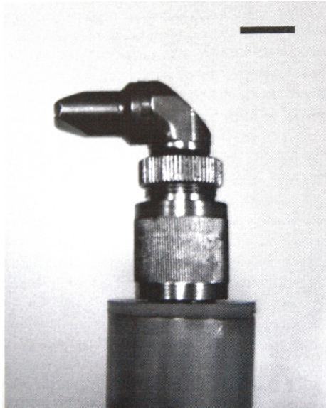
Figure 1.3: L-shaped tip of deflecting scanner 1.4 for examination of oral cavity. Bar = 1 cm
