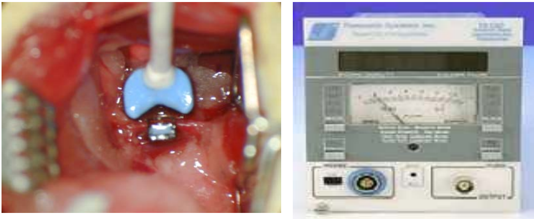
Figure 2: On the left, a perivascular doppler flow probe (Model 0.5 VB, Transonic Systems, Ithaca, NY) measuring flow on the right common carotid artery. On the right, a flowmeter (Transonic, Model T106) device.
