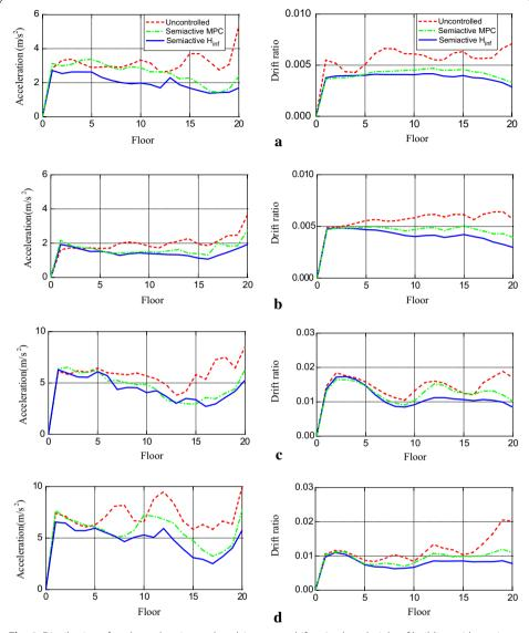
**Fig. 4** Distribution of peak acceleration and peak interstory drift ratio along height of building with semi-active H∞ control and without control subjected to different earthquakes. **a** El Centro; **b** Hachinohe; **c** Northridge; **d** Kobe
