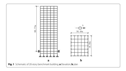
the assumption of Rayleigh damping. The first five natural frequencies of the twenty-story benchmark building are: 0.261, 0.753, 1.30, 1.83 and 2.40 Hz.
