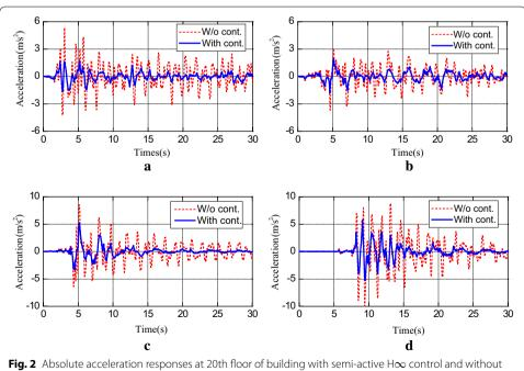
**Fig. 2** Absolute acceleration responses at 20th floor of building with semi-active  $H\infty$  control and without control subjected to different earthquakes. **a** El Centro; **b** Hachinohe; **c** Northridge; **d** Kobe
