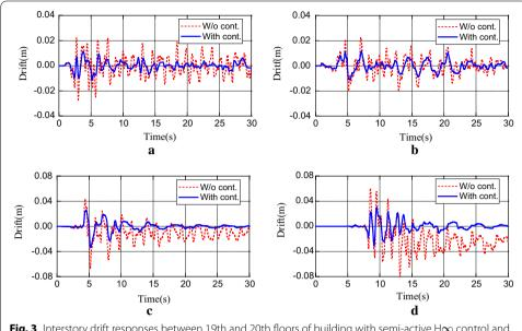
Fig. 3 Interstory drift responses between 19th and 20th floors of building with semi-active H∞ control and without control subjected to different earthquakes. a El Centro; b Hachinohe; c Northridge; d Kobe
