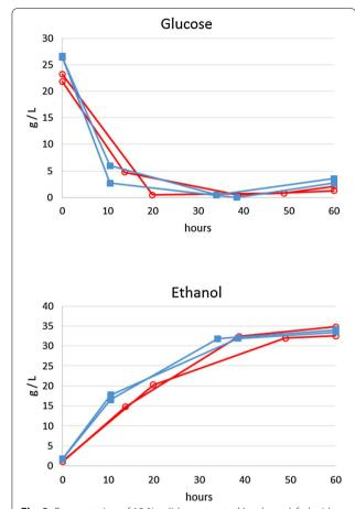
**Fig. 2** Fermentation of 12 % solids pre-treated hardwood, fed with hemicellulose extract. Duplicate 1 L fermentations with strain ALK2 are shown in *red* with *open circles* and with strain M2886 in *blue filled squares*
