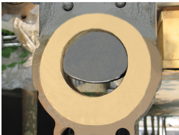
Fig. 1 Industrial application of ZTA ceramics as seal valves.
