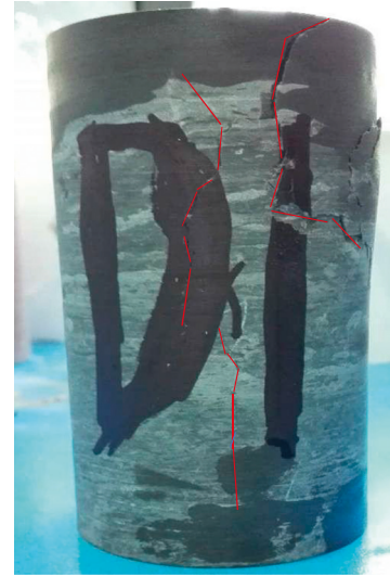
FIGURE 7: Schematic view of the shale rock specimen after failure.
