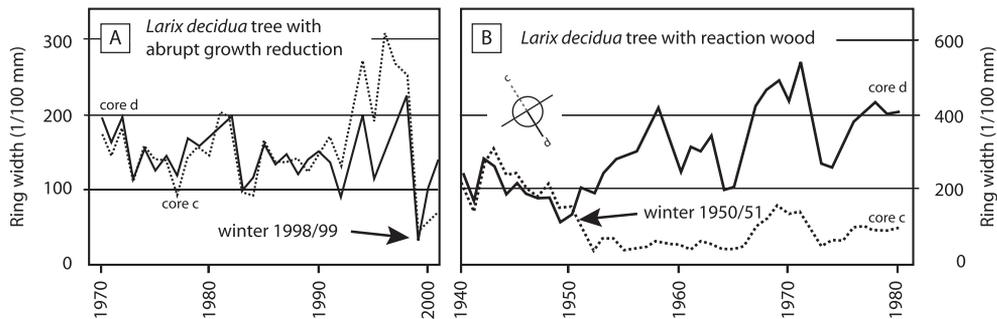
**Figure 5.** (A) Short, but abrupt growth reduction occurring as a result of damage caused during an avalanche in winter 1998/99; (B) after the tilting of the stem due to an avalanche in winter 1950/51, this tree started to produce reaction wood on the downslope side of the trunk (core d), whereas increment slightly dropped in core c (raw data: Hassler, 2004).
