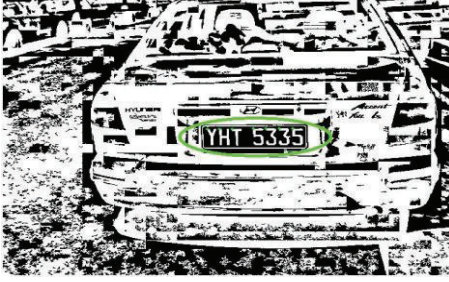
FIGURE 8: Resultant image after thinning and resizing technique.
