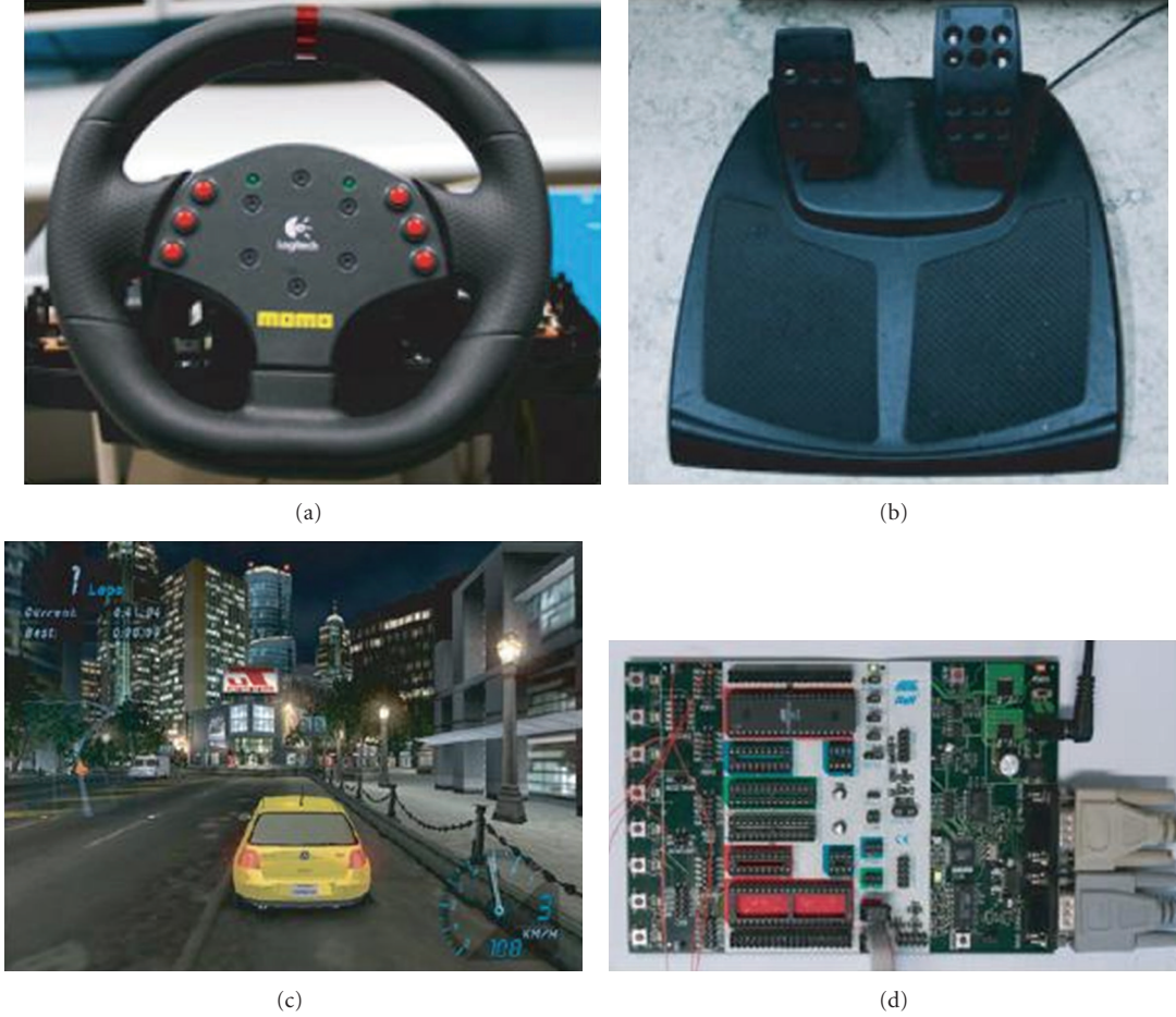
FIGURE 4: (a) Steering wheel; (b) Acceleration and brake pedals; (c) Simulated driving scene; (d) Processor circuit board.
