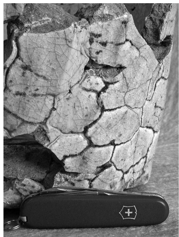
Fig. 5. Side of the crucible close to flame. Note the crack network on the surface due to thermal stress.
