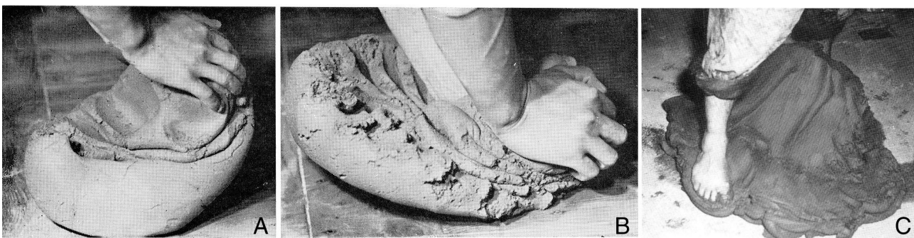
Figure 3.1: A, B: kneading with the hands (SANDERS, 1976) and C: with the feet (RADA, 1991).
