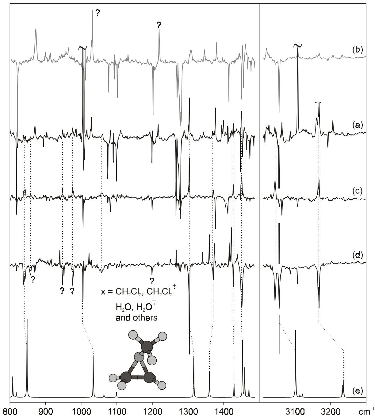
Figure 4-24: IR difference spectra of NMA (a) after (45 min.) and (b) (180 - 45 min.) X-irrad.; (c) after 45 min. irrad. at >475 nm and (d) after 40 min. >420 nm. (e) spectrum of \text{NMY}^{\ddagger} calculated on B3LYP/6-31G* level, all frequencies scaled by a factor of 0.96.
