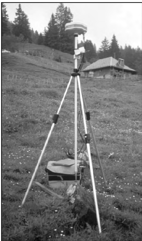
Fig. 3.1 GPS mobile station at the Hohberg landslide (point 13; Ann. 8).
