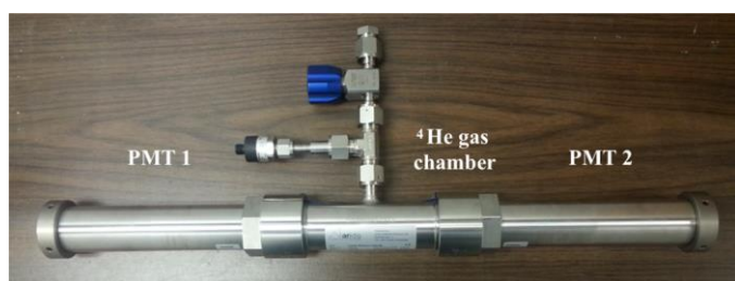
Fig. 1. A PMT based Helium-4 fast neutron detector. The active volume at the center is pressurized to 150 bar.
