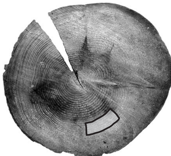
Sample Ho43, arising from the Hohberg landslide Number of tree-rings: 54 Radiocarbon dated tree-rings: 19 to 25, mean: 22 Radiocarbon age: 1180 \pm 20 BP Calibrated age: 1180-1010 cal BP Correction of radiocarbon age: subtract 32 to calibrated age Corrected age: 1148-978 cal BP
