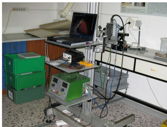
Fig. 2 The portable XRF instrument used for the surface, non-invasive analysis
