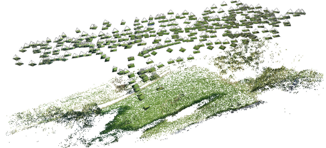
Figure 7. Sparse reconstruction result of Set1 showing the sparse point cloud and the camera poses.
