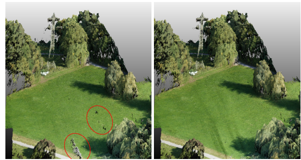
Figure 15. Comparison of 3D reconstruction: The left image shows the reconstruction without filtering the power lines and the right image the reconstruction with filtered power lines. It is clearly visible that filtering the power lines removes reconstruction artefacts like spikes toward the power line (marked by red ellipses).
