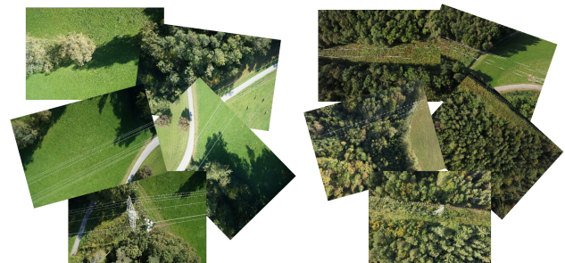
Figure 5. Comparison of acquired image sets. The differences in resolution (see power pylon) and the changes in season are visible.
