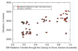
FIG. 12. Relations of shortwave radiative (through plant canopy to snowpack) transfer coefficients to elevation, in the Merced River model (above Happy Isles Bridge), before and after adjustments for seasonal-mean cloud cover, spring 1999.
