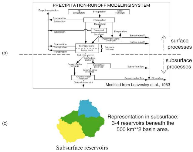
FIG. 11. The U.S. Geological Survey's PRMS, with details for the Merced River model.
