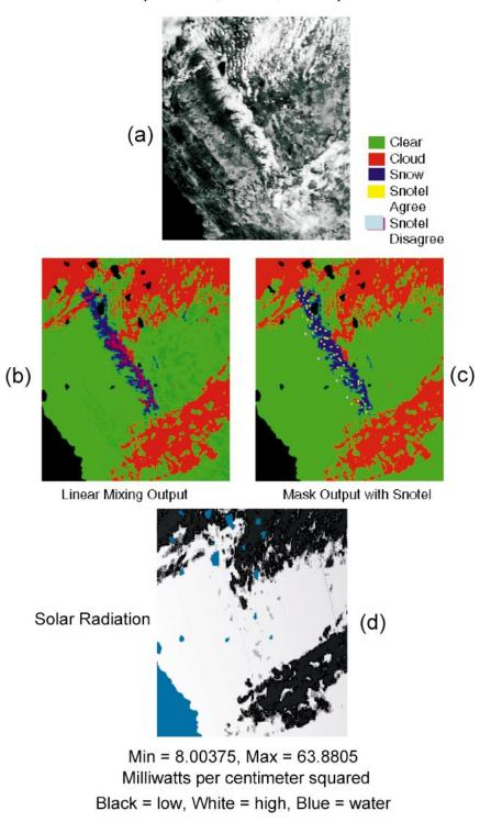
FIG. 3. (a) GOES broadband visible data for 19 Apr 1999. The area imaged corresponds to the dashed box in Fig. 1. (b) The RNNCCS-linear mixing model classification. (c) The RNNCCS discrete classification with snowpack telemetry-instrumented validation (SNOTEL) sites shown. (d) Insolation reaching the ground based on satellite-detected cloud cover. See text for details.
