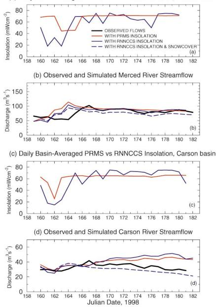
FIG. 15. Similar to Figs. 13a and 13b but for simulations of streamflow in the Merced and Carson Rivers during a part of Jun 1998. See the text for details.
