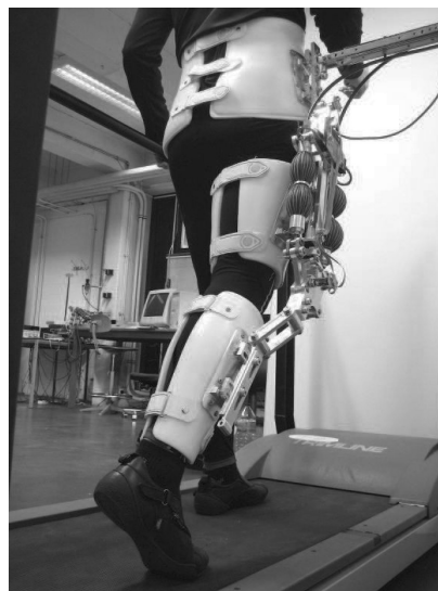
Figure 1. Close up of the unilateral exoskeleton with the knee joint powered by pleated pneumatic artificial muscles.
