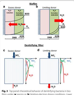
films under (**a**) excess or (**b**) limiting electron donor conditions. *Lower* panels theoretical nitrogen profiles in a denitrifying filter in presence of (**c**) excess or (**d**) limiting electron donor
