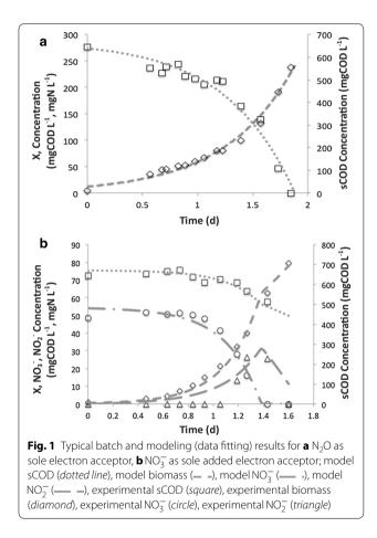
$NO_3^-$  reduction test. The Y for reduction of  $NO_2^-$  to  $N_2O$ , in gCOD/gCOD, was assumed to be the same as the Y for reduction of  $N_2O$  to  $N_2$  (Hiatt and Grady 2008; Ni et al. 2011).
