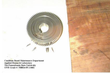
(b) Five fully broken and two partially broken teeth
