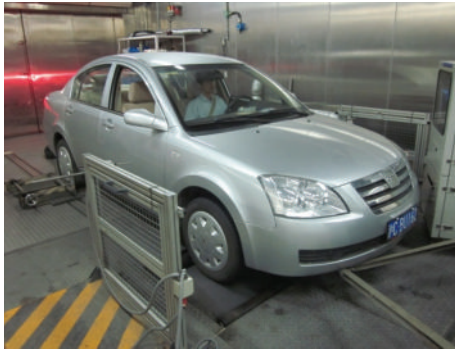
FIGURE 10: Five-speed dry DCT real vehicle chassis dynamometer test.
