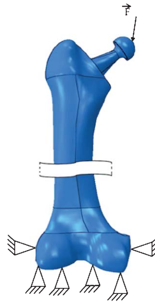
Fig. 4. Boundary condition showing the force vector acting on the head and the fixation of the distal epiphysis.
