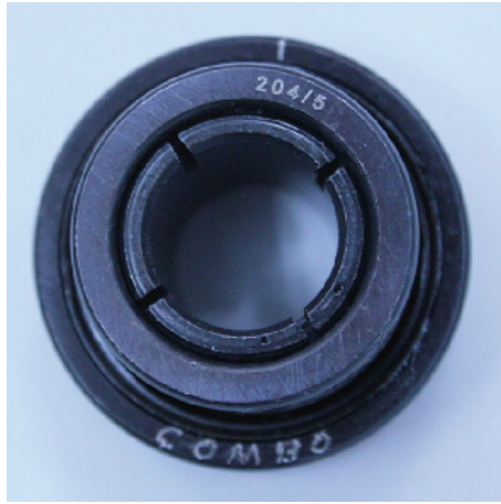
(a) A bearing with compound faults
