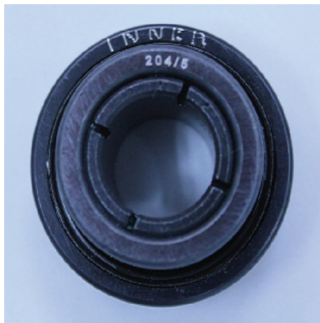
(c) A bearing with inner race fault
