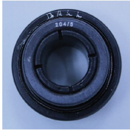
(b) A bearing with rolling element fault
