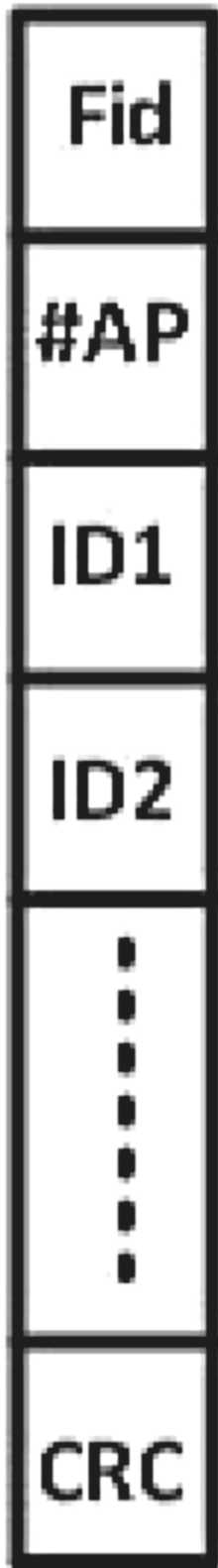
Fig. 6 Metadata structure. This is the metadata that is transmitted with CF-Poll frames
