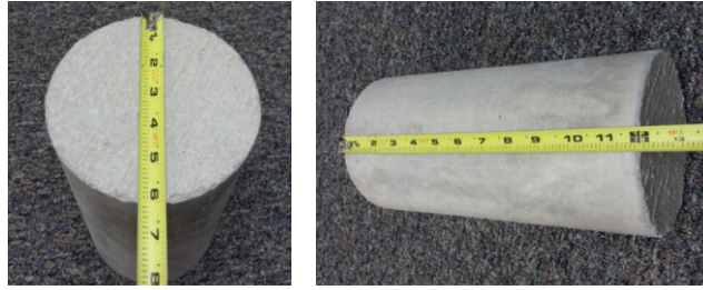
FIGURE 25: The concrete cylinder used for the experiment. Measured dimensions are in inches.
