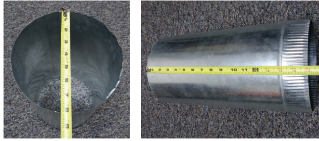
FIGURE 16: The metallic cylinder used for the experiment. Measured dimensions are in inches.
