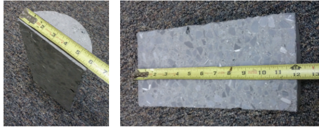
FIGURE 31: The semicircular concrete cylinder used for the experiment. Measured dimensions are in inches.
