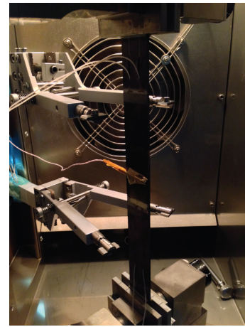
FIGURE 4: A sample of CFRP in testing machine.
