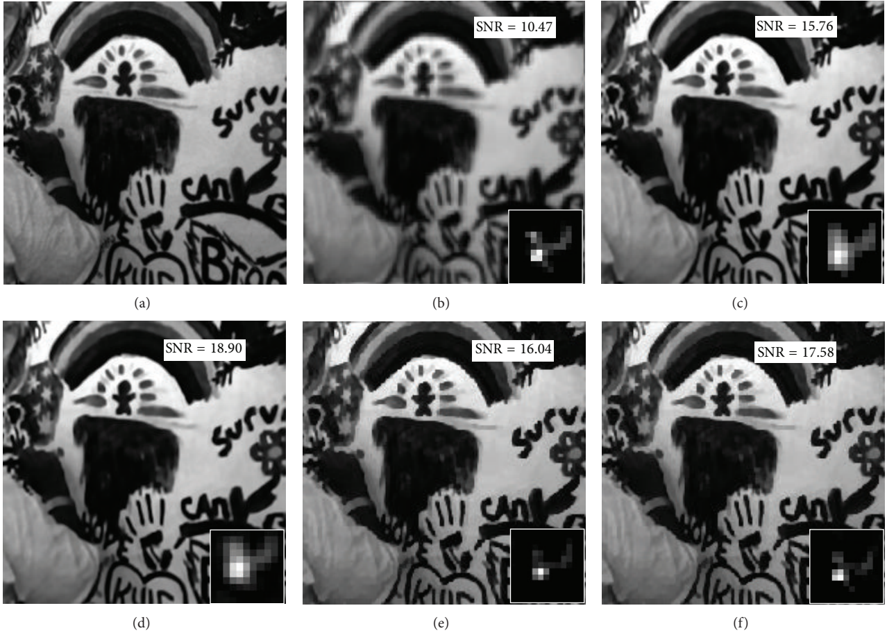
FIGURE 7: Estimated PSFs and corresponding restored images by different algorithms. (a) The clear image. (b) Blurred image and the degrade PSF. (c) The result of Fergus et al.'s method in [13]. (d) The result of Levin et al.'s method in [15]. (e) The result of Hu et al.'s method in [16]. (f) Our result.
