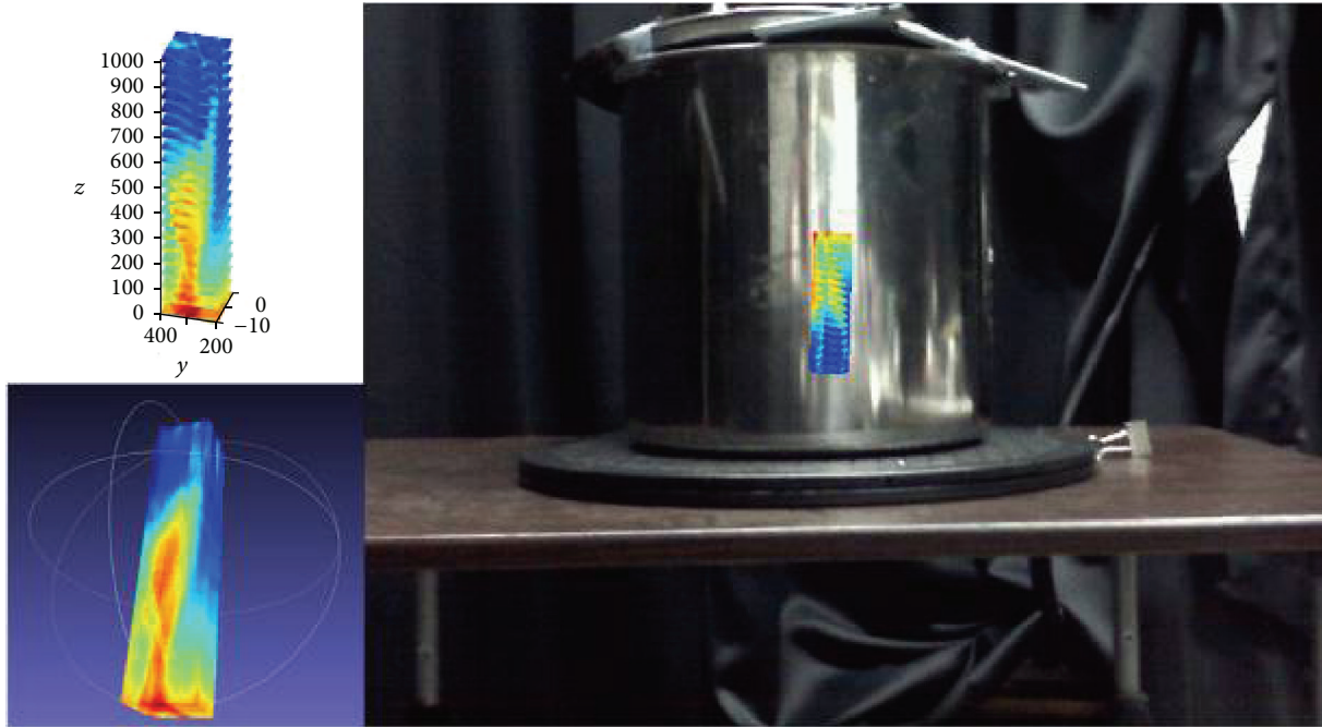
FIGURE 7: A metal container and the reconstructed 3D model with thermal mappings.
