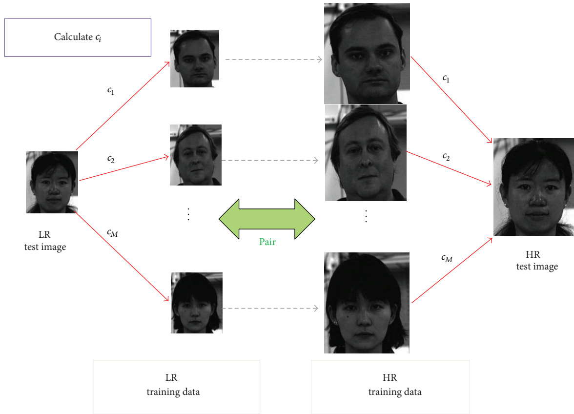
FIGURE 1: Schematic diagram of face hallucination.
