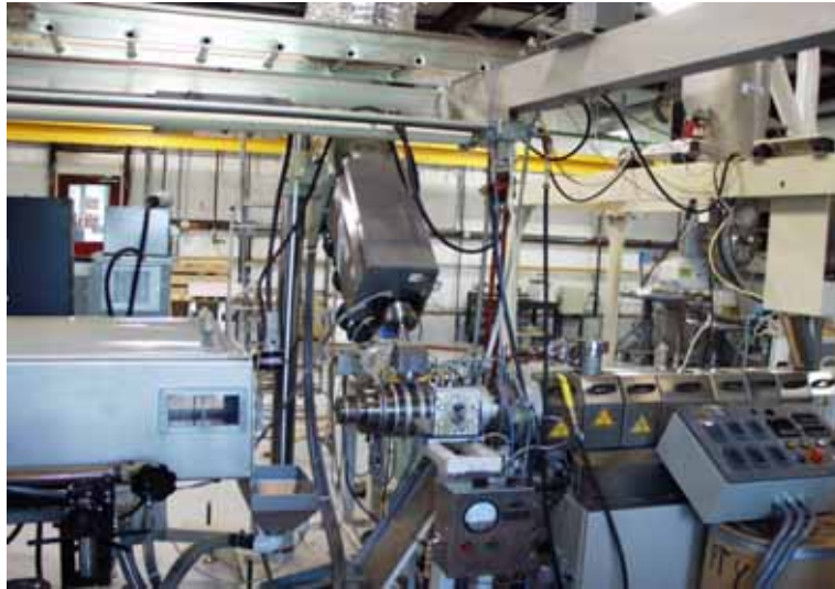
FIGURE 1. Main part of the extrusion setup. From right to left: the 40-mm twin screw extruder with a die at the end, the co-extruder at 45 degrees above the extruder, and the vacuum cooling tank.
