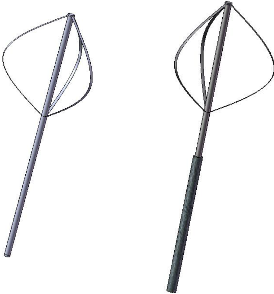
Figure 4.4.4 Drawing of the two main concepts: a. “all steel structure” b. steel structure with concrete foundation
