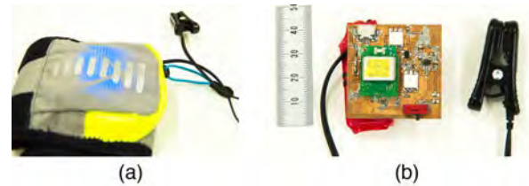
Fig.1. (a) Overview of the wearable device in a sports wrist pocket (b)the circuit board and heart pulse sensor
