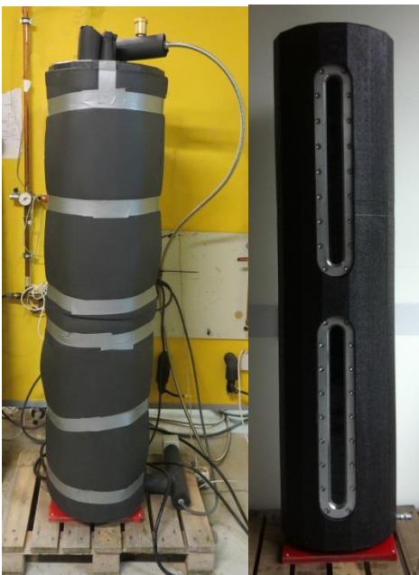
Figure 1a and 1b. The Thermobatterie test setup and tank with inspection windows.
