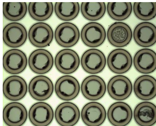
Fig., 2: Top view of an array of micro wells filled with dried furosemide solution
