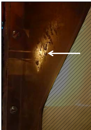
Figure 83 – Particle void with low particle concentration in the entrainment area. Point of interest is marked by arrow.
