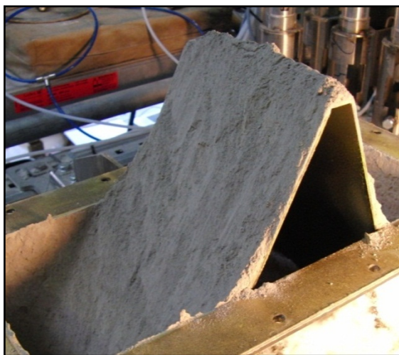
Figure 94 – Side view of the interior of the bottom stage after the PoC experiments, showing particle outlet #1
