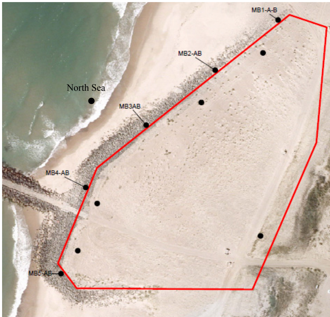
Figure 4. Placement of the monitoring wells (MB1-5) at the foreshore immediately down-gradient of the sheet pile barrier. Also, the approximate location of the most frequent sampling point in the North Sea.
