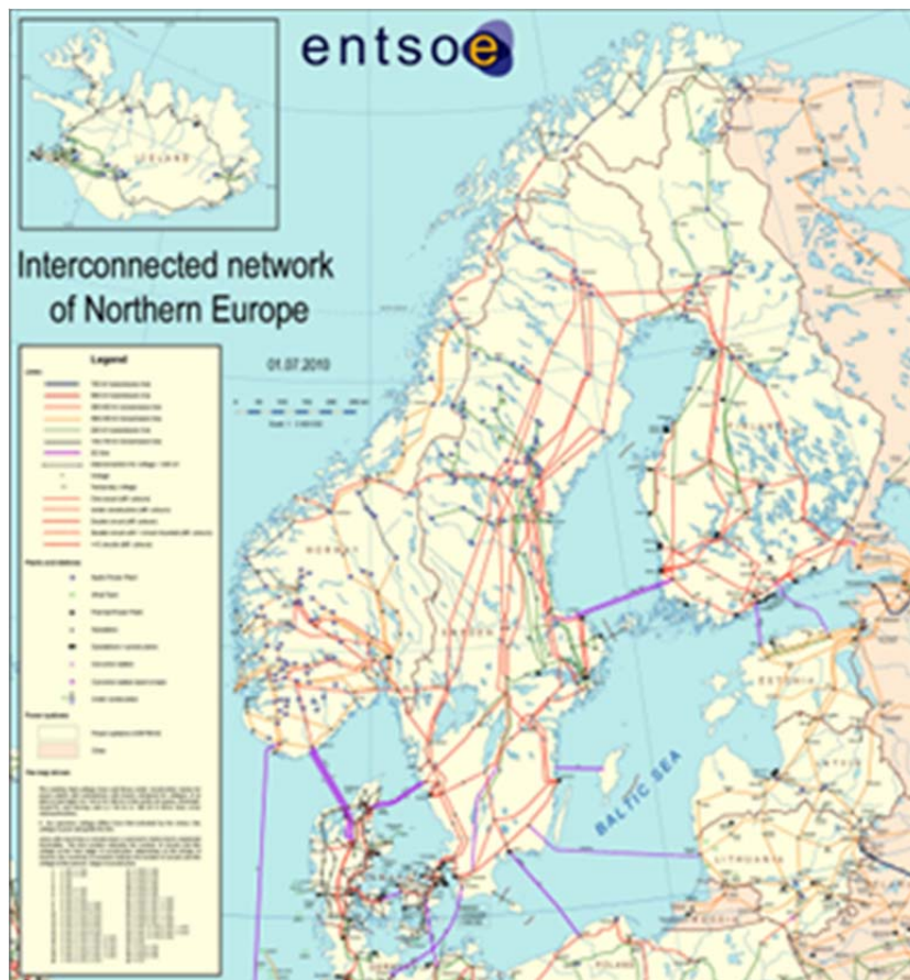
Fig. 1. The interconnected high voltage transmission grid in northern Europe[3].
