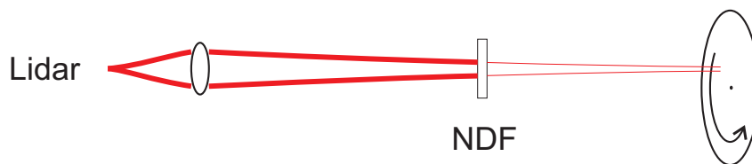
Figure 3. Schematic drawing of the setup used to measure the SNR from a moving hard target. The neutral density filter (NDF) attenuates the laser beam by 25 dB upon each passage.
